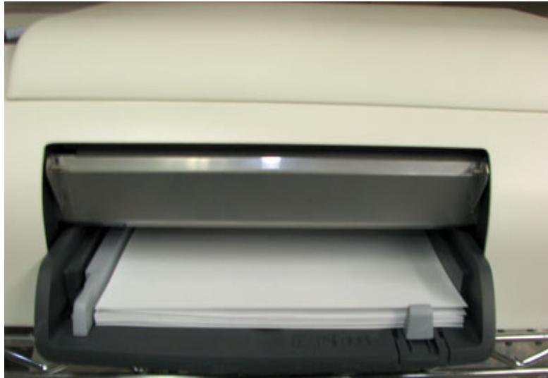
Shows the input tray in the front of the embossing printer
