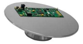
Tilt table includes 2 different heights that can be used with +3 or +4 lens, depending of the height of you object.
