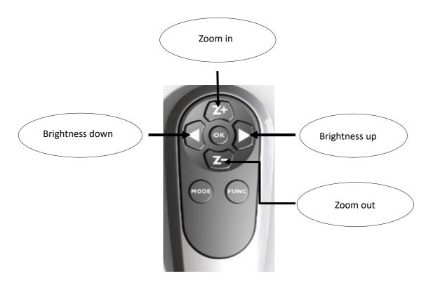
**Z+** Zoom in. **Z -** Zoom out.  $\triangleright$  Increase brightness.  $\triangleleft$  Decrease brightness. Press **Func** short and autofocus will go off / on. When autofocus is off,  $\triangleleft$  &  $\triangleright$  will change functions to adjust focus as a manual focus. **OK** change magnification to wide and show an artificial cross. Next press on **OK** the magnification goes back to previous magnification. A quick press to **Mode** camera will change between color and greyscale.
